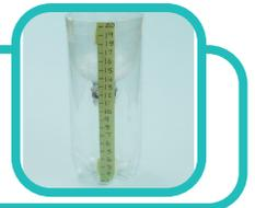
5 Dig a hole and bury your rain gauge so that the top is sticking about 5cm out of the ground. This will stop the rain gauge from blowing down on windy days.
