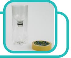
3 Make a scale in centimetres on a piece of tape, using a ruler, and fix it to the side of your bottle. You could sellotape a spare ruler on the side if you have one.
